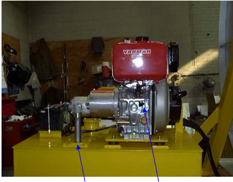
Suction Pipe / Throttle Control
