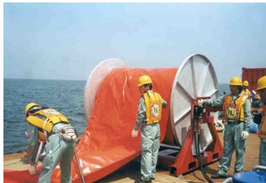
The PAJ team deploys the Deep Sea Inflatable boom off the deck of a Japanese vessel in the Ise Wan Sea.
