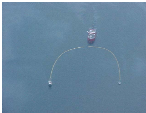
Overhead shot of the VALDEZ STAR in action collecting spilled diesel oil in Northern Prince William Sound.
