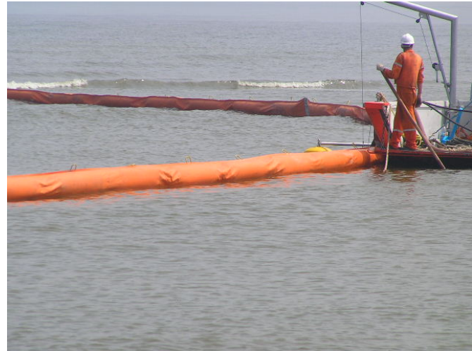
Slickbar's Mk E General Purpose Oil Spill Containment Boom being used to coral oil along the beach operations of the exercise.
